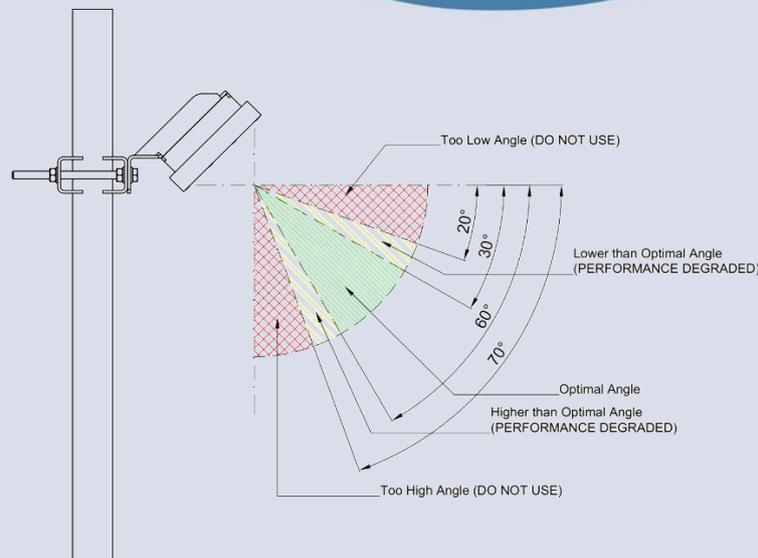
The instrument is equipped with internal inclination angle sensor. The measured inclination (tilt angle) is reported by the instrument and can be seen in the PC application for instrument configuration. It is strongly recommended to check the inclination measured by the instrument itself during equipment installation. This measurement is also used internally for automatic velocity cosine compensation.
