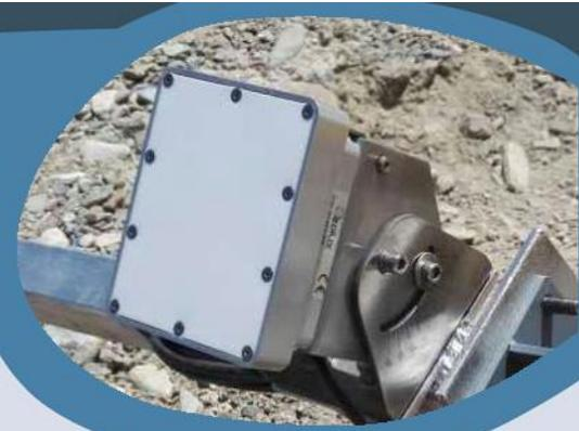
In both directions, so for such sites, the radar sensor should be configured to report both incoming and outgoing flow, by selecting “both direction” setting in the radar sensor.
